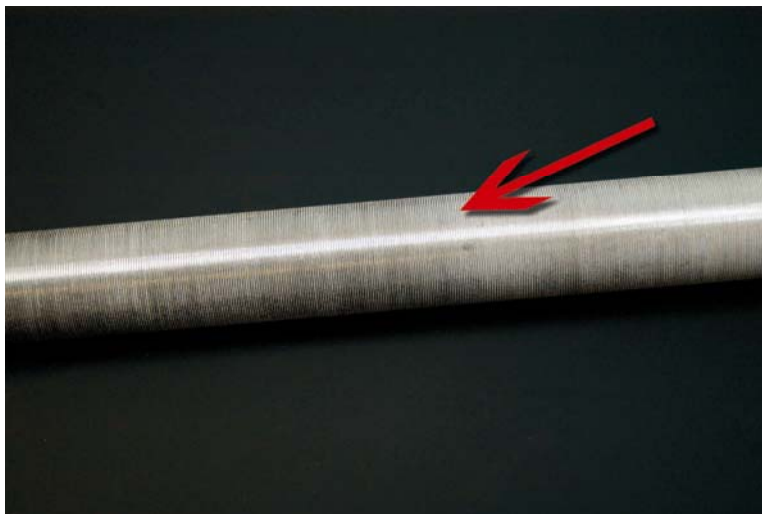
Example of coating roller with oxidation that should be replaced.
